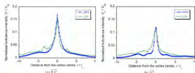
Figure 19: Comparison of turbulence measurements using DPIV and LDW: (a)  $\overline{V_r^2}$ , (b)  $\overline{V_z^2}$ .
