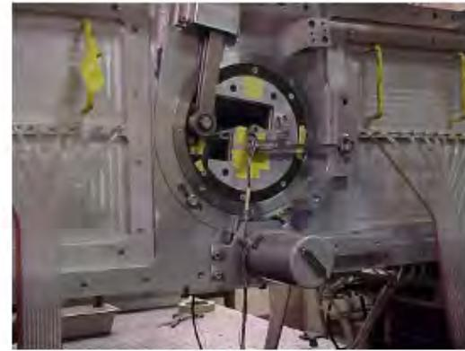
VDLE airfoil in CDSF, with drive linkage set for variable droop
