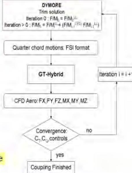
Figure 3 LC methodology between GT-Hybrid and DYMORE
