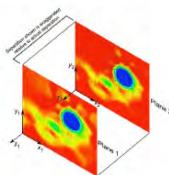
Figure 4: Typical instantaneous velocity fields measured using DPS-DPIV. Interplane separation is exaggerated; actual plane separation is much smaller than vector-to-vector spacing within each plane.
