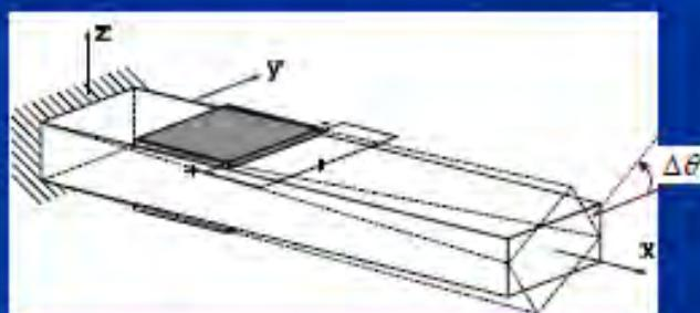
Schematic of ATR via induced shear actuation
