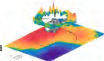
*Bo105 rotor: pressure fluctuations and contour noise levels (DNW experiment)*
