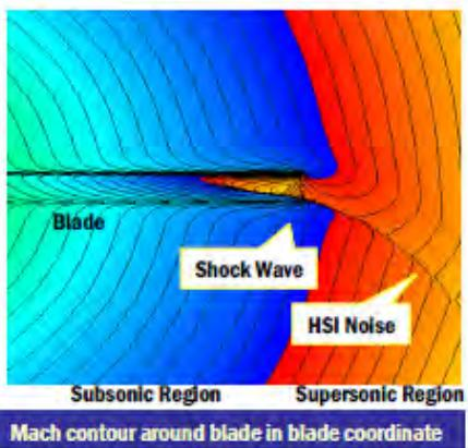
Mach contour around blade in blade coordinate
