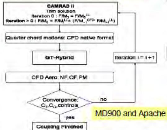
Figure 2 LC methodology between GT-Hybrid and CAMRAD II
