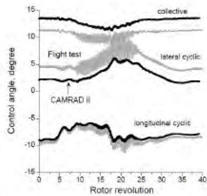
Fig. 8 (a) Rotor blade control angles
