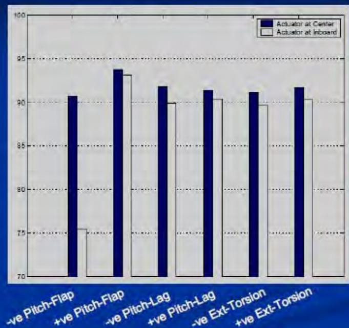
Unlike high speed case, actuator at center shows better performance than that at inboard.
