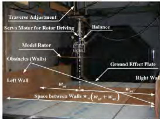
Figure 1. General View of the Experimental Facility
