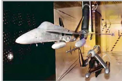
**Grid Survey test within flow field of the 6% CF-18 stores model**
