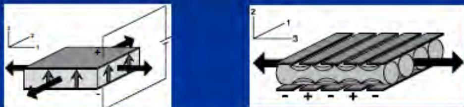
**d<sub>31</sub> actuation** ← normal strains → **d<sub>33</sub> actuation**
