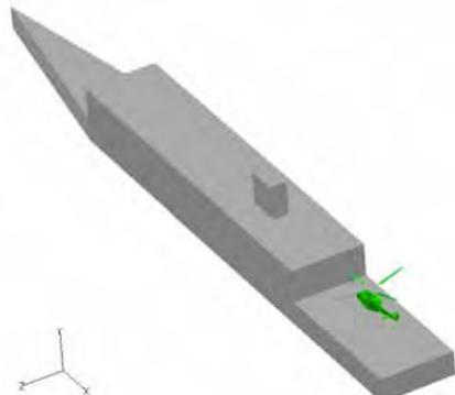
(2) Bell 412 helicopter landing on ship-deck in the environment of ship airwake
