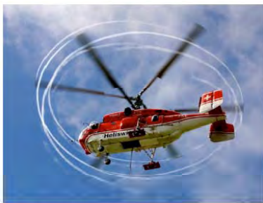
Figure 1: The blade tip vortices from a coaxial rotor helicopter rendered visible by natural condensation and showing the interference between the rotors.
