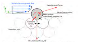
Figure 2: Forces acting on sediment particles at rest beneath a boundary layer flow.
