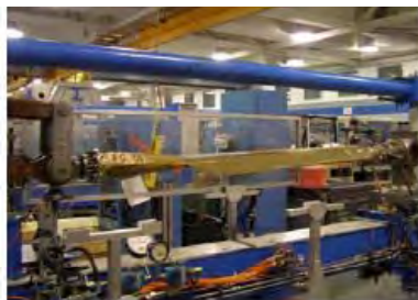
Figure 8. Fatigue test of main rotor blade root end.
