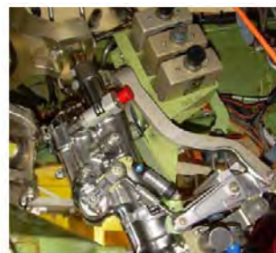
Figure 11. Demonstrator main rotor fly-by-wire servo installed in the aircraft.
