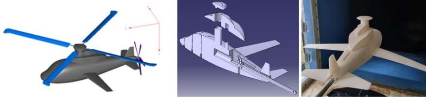
▲ Wind tunnel experiments for HCUR scaled model
