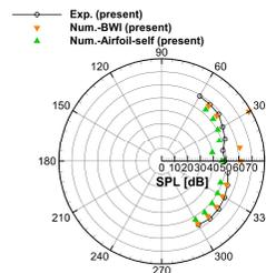
Rotor noise prediction for a 3-bladed UAV rotor
