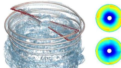
Coaxial, counter-rotating rotor
