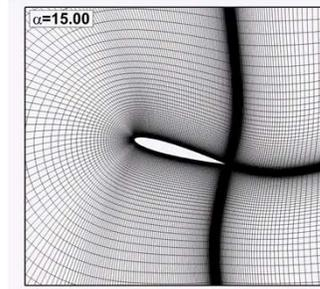
▲ Dynamic stall prediction by using RBF-based grid deformation
