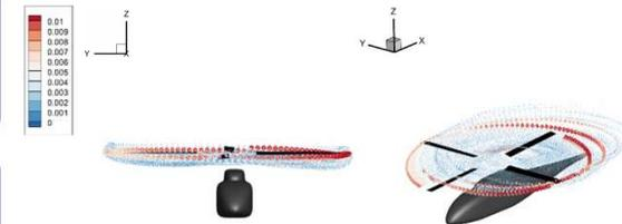
NVLM/VPM/CFD simulation of complete rotorcraft
