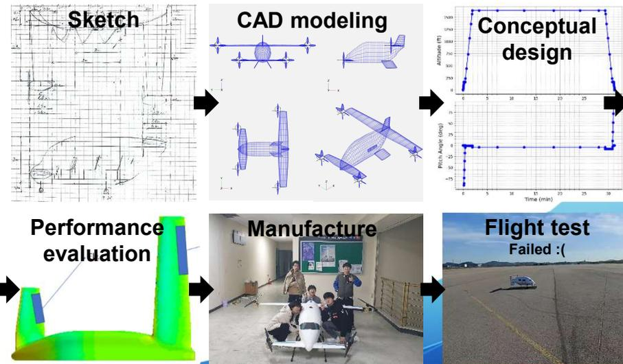
Design, manufacture, and flight test of a tilt-rotor UAM vehicle
