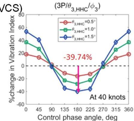
Active vibration control for medium utility helicopter using Higher Harmonic pitch Control
