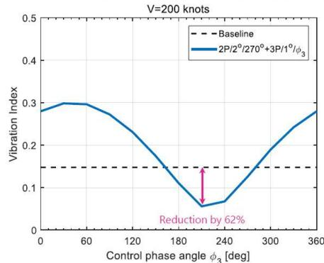
Active vibration control for X2TD rotor using Individual Blade pitch Control
