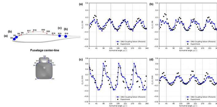
Fundamental formulation and validation results of NVLM/VPM/CFD simulation
