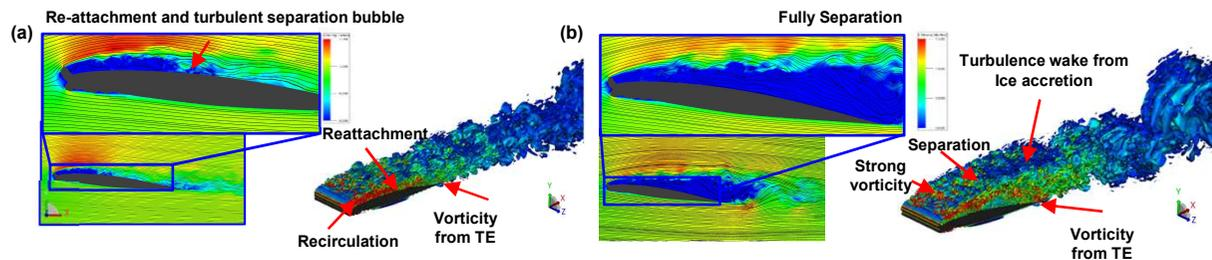
Instantaneous x-velocity contour and  $\lambda_2$  iso-surface: (a) 6 deg. (b) 8 deg.
