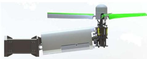
TiltRotor Aeroelastic Stability Testbad (TRAST, US)
