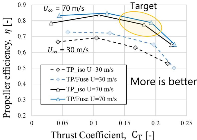
Thrust – efficiency (w/&w/o Fuselage)
