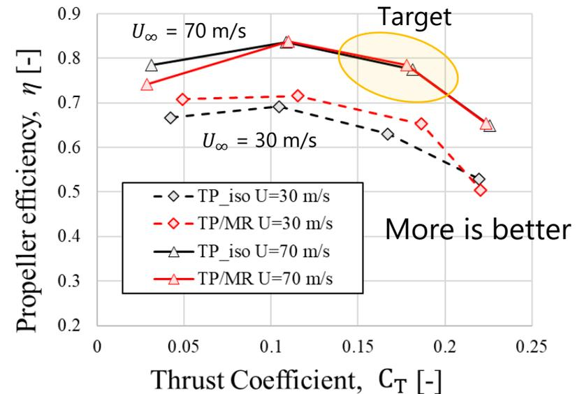
Thrust – efficiency (w/&w/o Main rotor)
