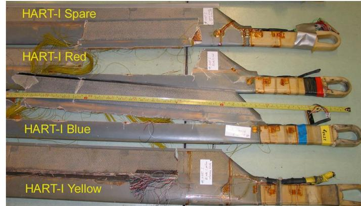
HART I blades used for structural test
