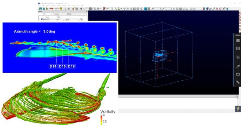
3D compressible RANS flow solver **KFLOW**
