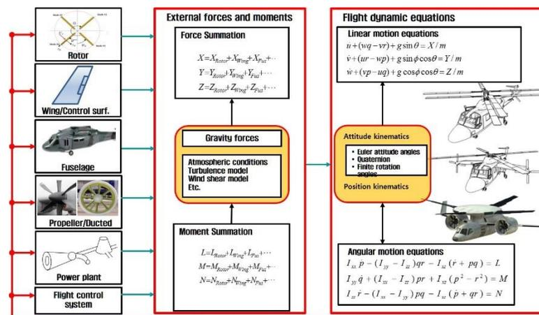
Rotorcraft flight dynamics simulation S/W **HETLAS**
