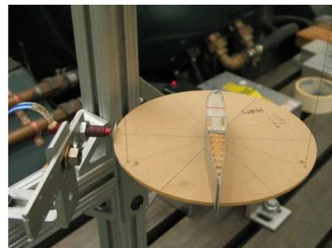
Trifillar pendulum for section MOI
