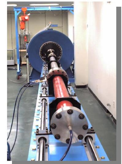
High speed shock tube (M = 2.5)
