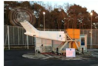
Figure 29. The ETR machine running on the iron bird rig
