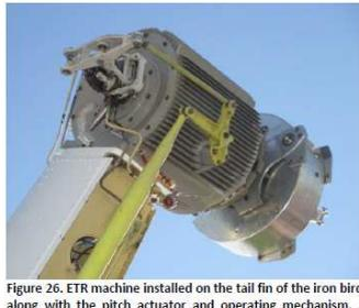
Figure 26. ETR machine installed on the tail fin of the iron bird, along with the pitch actuator and operating mechanism. A hub equivalent mass is fitted to the ETR shaft in preparation for resonance testing
