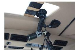
Figure 3: Smartcam as installed on R66.
